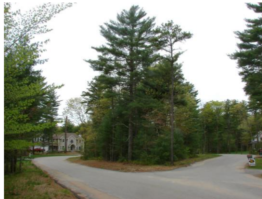
Figures 17 and 18 When the above concept is not feasible, cul-de-sacs should at least be terminated with an island planted with canopy shade trees to properly fill the “celestial space” above this wide bulbous street form. Or existing trees can be left in place. Plowing snow is much easier because plow operators can make one efficient sweep around the central island.
