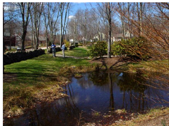
Fig. 11 Swales can easily serve in place of curbs, even when density is more than two or three dwellings per acre.
