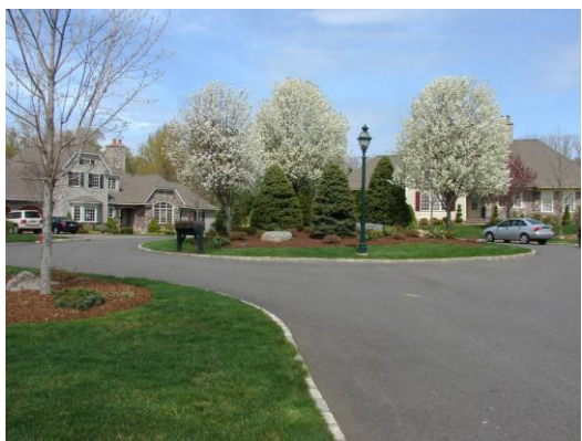
Figures 17 and 18 When the above concept is not feasible, cul-de-sacs should at least be terminated with an island planted with canopy shade trees to properly fill the “celestial space” above this wide bulbous street form. Or existing trees can be left in place. Plowing snow is much easier because plow operators can make one efficient sweep around the central island.
